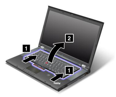
8. Carefully lift the keyboard until you can see how it is connected. Hold the keyboard above the computer, and then detach the connector. Remove the keyboard.
